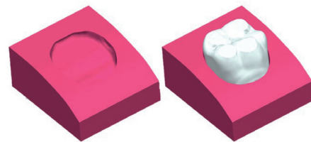
Fig. 4. Design images of the resin block for fracture load resistance test. Left: image of the resin block, right: image of the tooth placed on the resin block.
